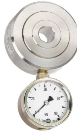
Hydraulic ring force transducer, model F6116
